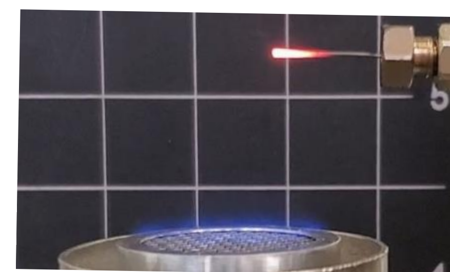
Capillary sampling from FPDSF with water droplets for GC/MS
