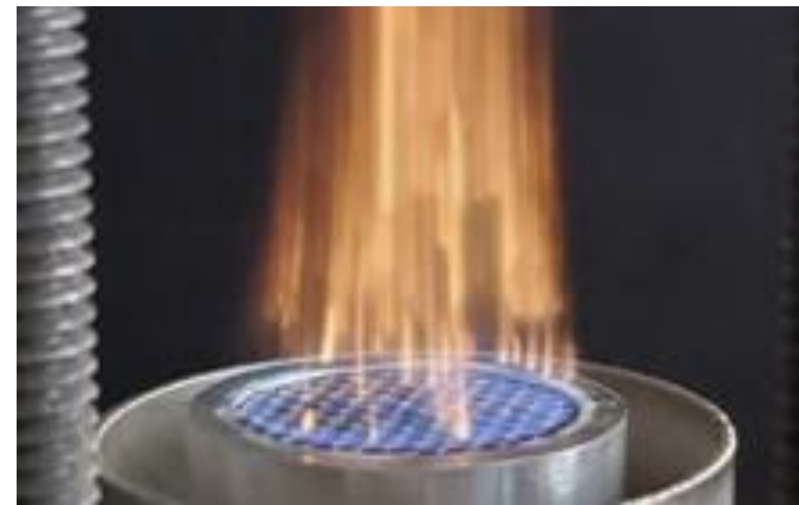
FPDSF seeded with monodisperse droplets of a 4% w Ni(NO 3 ) 2 water solution
