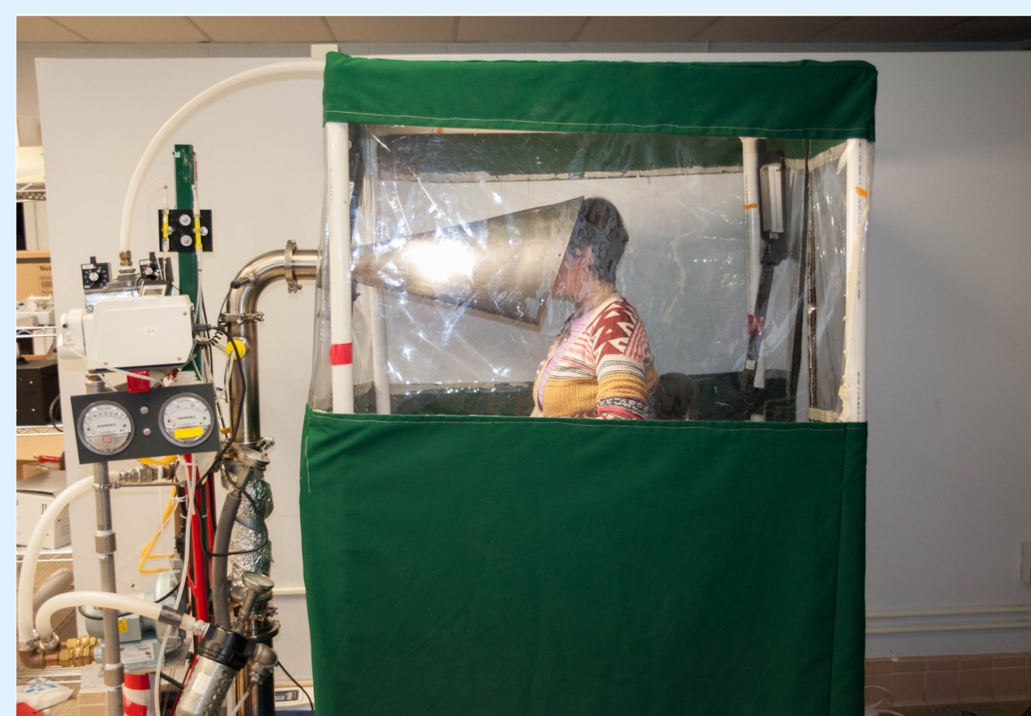
Figure 1. Gesundheit-II (G-II) exhaled bioaerosol collector
