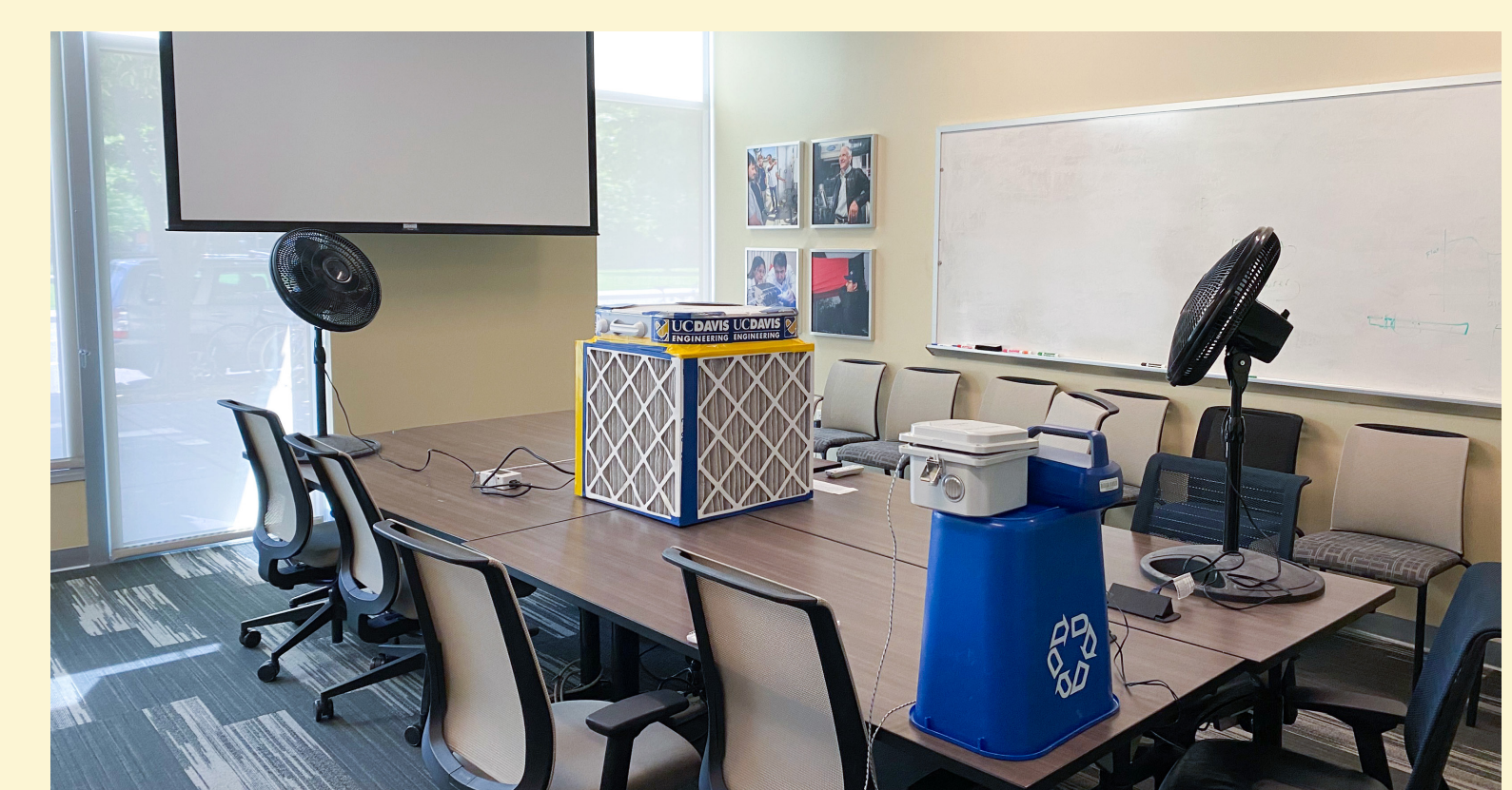
Example air cleaning test setup. CR box placed in center of room, and fans mix air during particle generation.
