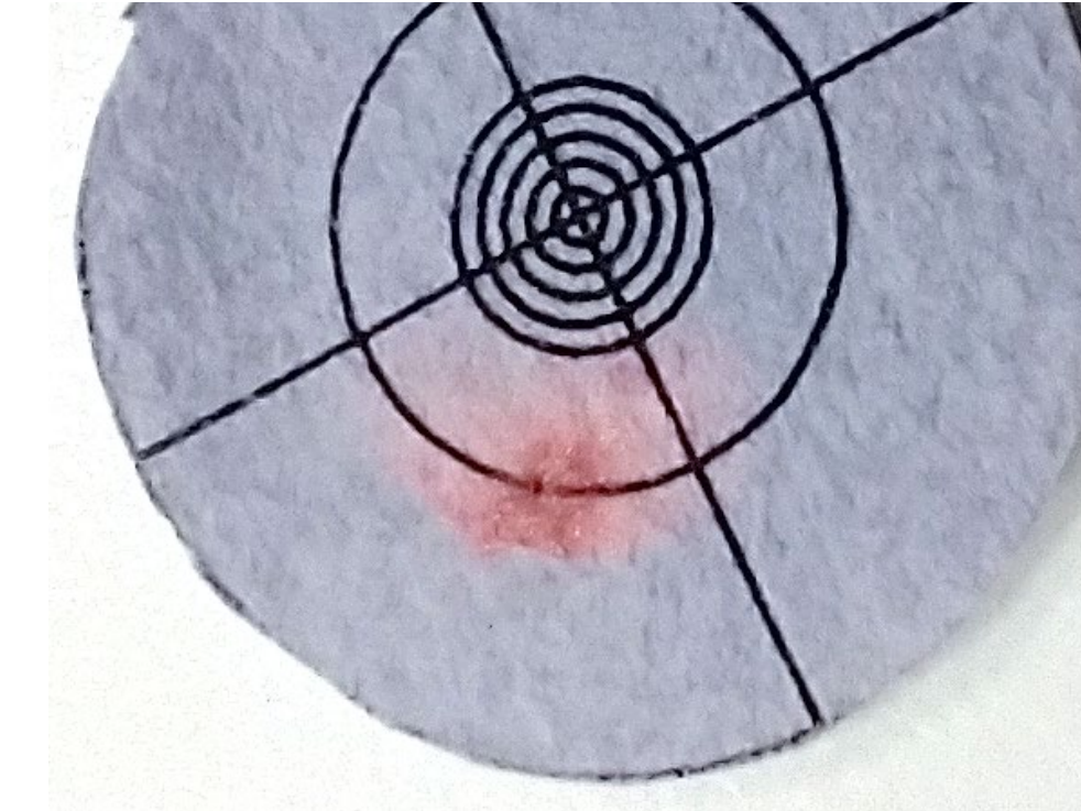
Photo of a litmus paper target post-test. The liquid deposited from the AS has changed color indicating it is acidic.
