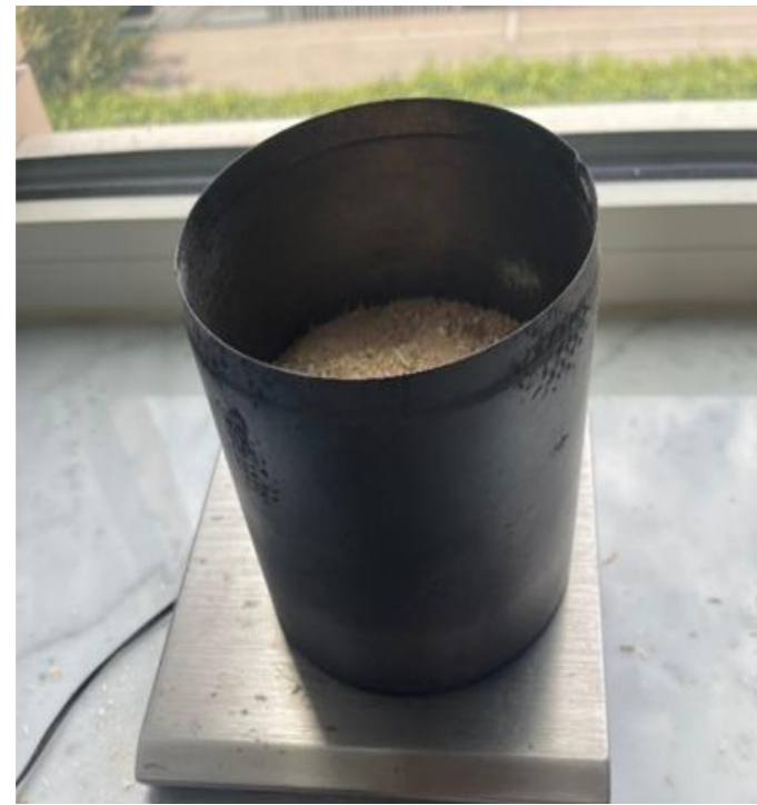
Wood sawdust undergoing slow pyrolysis
